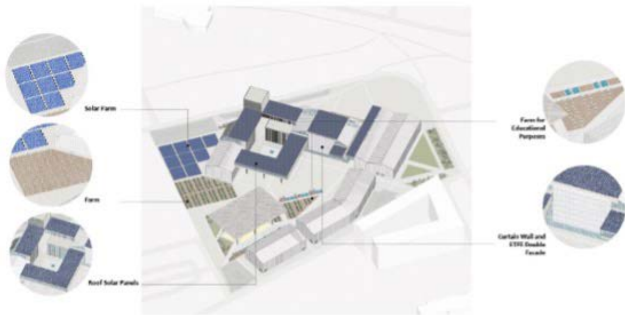
Figure 5: Diagram showing some of the sustainable design features included in the project. Image credit: Haya Al-Bayti, 2023.
